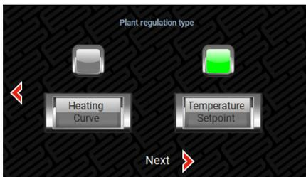
Next, you need to set the heat pump control method. There are two modes: heating curve and temperature setting.
