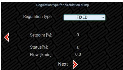
In addition, the control mode is selected. “Delta” ensures that a temperature difference of 5K is maintained between the inlet and outlet water temperatures of the exchanger, while “Fixed” gives you the option to set a constant flow rate.
