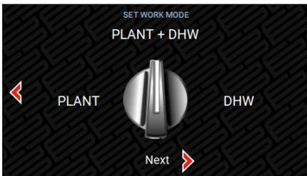
Once the compressor crankcase is warmed up, select the mode in which the heat pump will operate. There are three modes to choose from:
