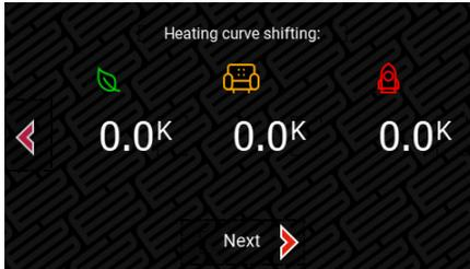
For the “temperature setpoint” mode, the CH temperature setpoints for Economy, Comfort and Pre-Comfort modes are set directly. Then, for both the “heating curve” and “temperature setpoint” modes, three fixed hot water temperature setpoints are set.
