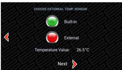
The next step is to select the temperature sensor that will be the master sensor in the control algorithms.
